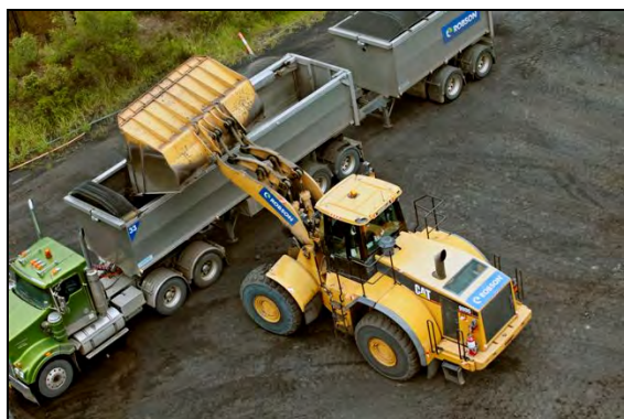
Plate 4-19 – Loading of ROM Coal into a B-Double Truck at the Tasman Underground Mine
