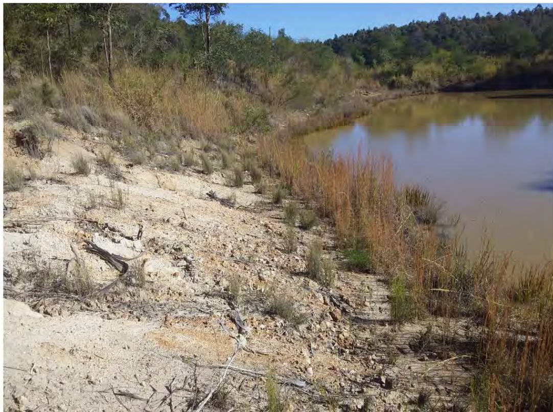
Photograph 2 Potentially Dispersive Soils around Foreshore of Sediment Dam D
