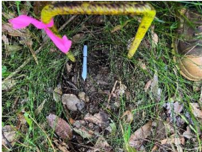
Plate 9: Quadrat 8 showing animal burrow under the H frame negating the soil loss measurement
