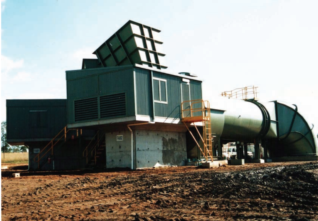
Illustration 10: Photograph of the type of ventilation shaft proposed for the underground mine.
