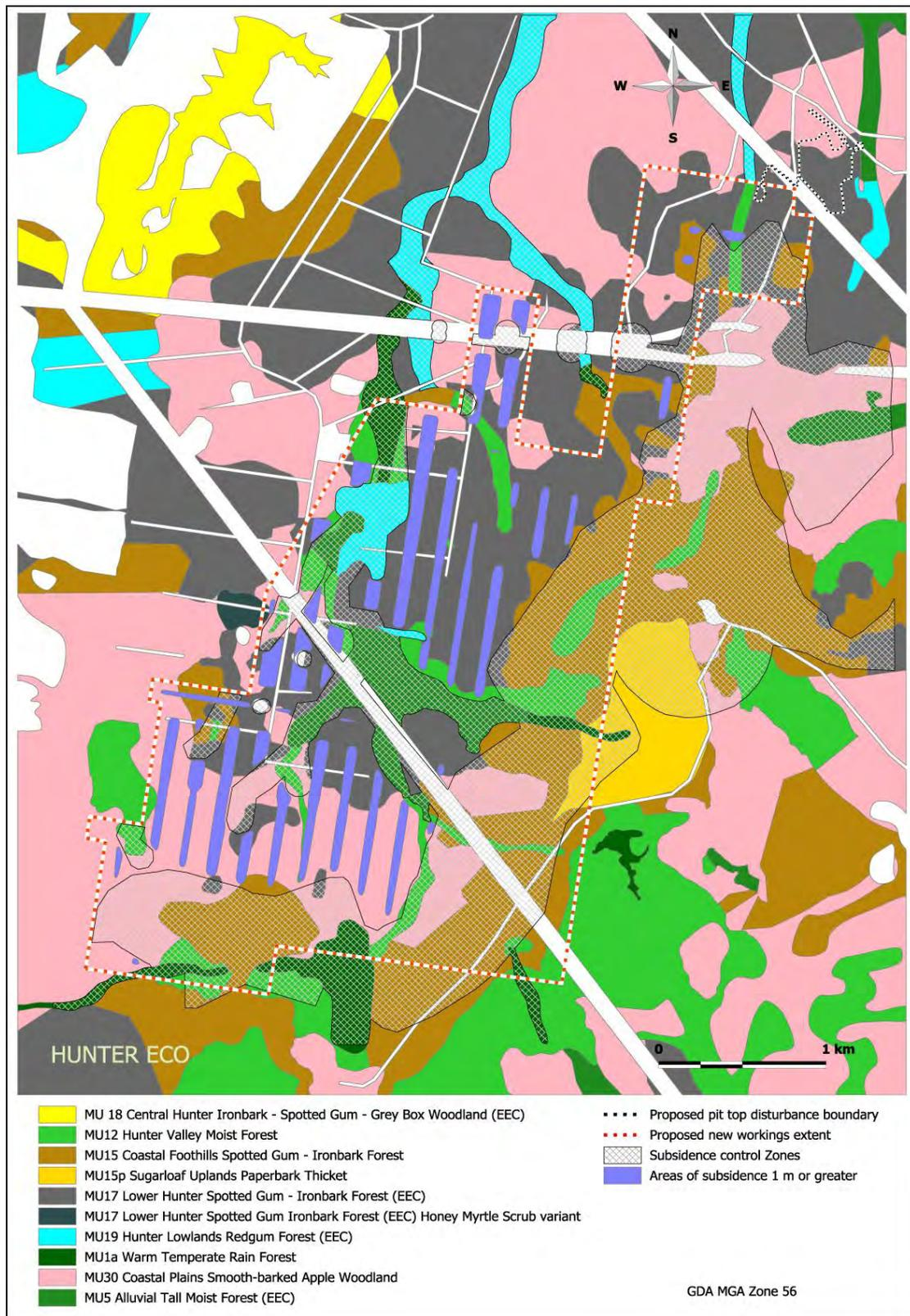
**Figure 6 Proposed subsidence control zones and maximum subsidence zones**
