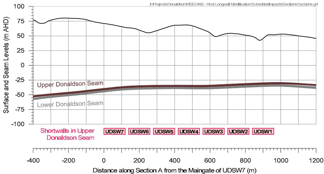
**Fig. 1.2 Surface and Seam Levels along Section-A (Shortwalls in Upper Donaldson Seam)**
