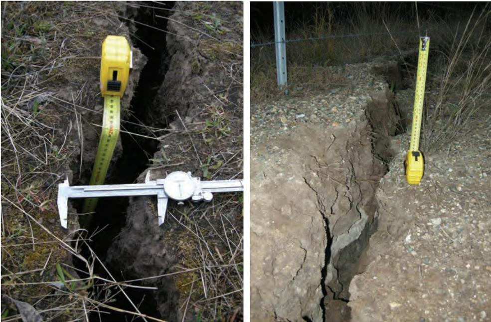
**Fig. 4.4 Photographs of Typical Surface Cracking in the Hunter Coalfield (Less than 100 metres Depth of Cover)**
