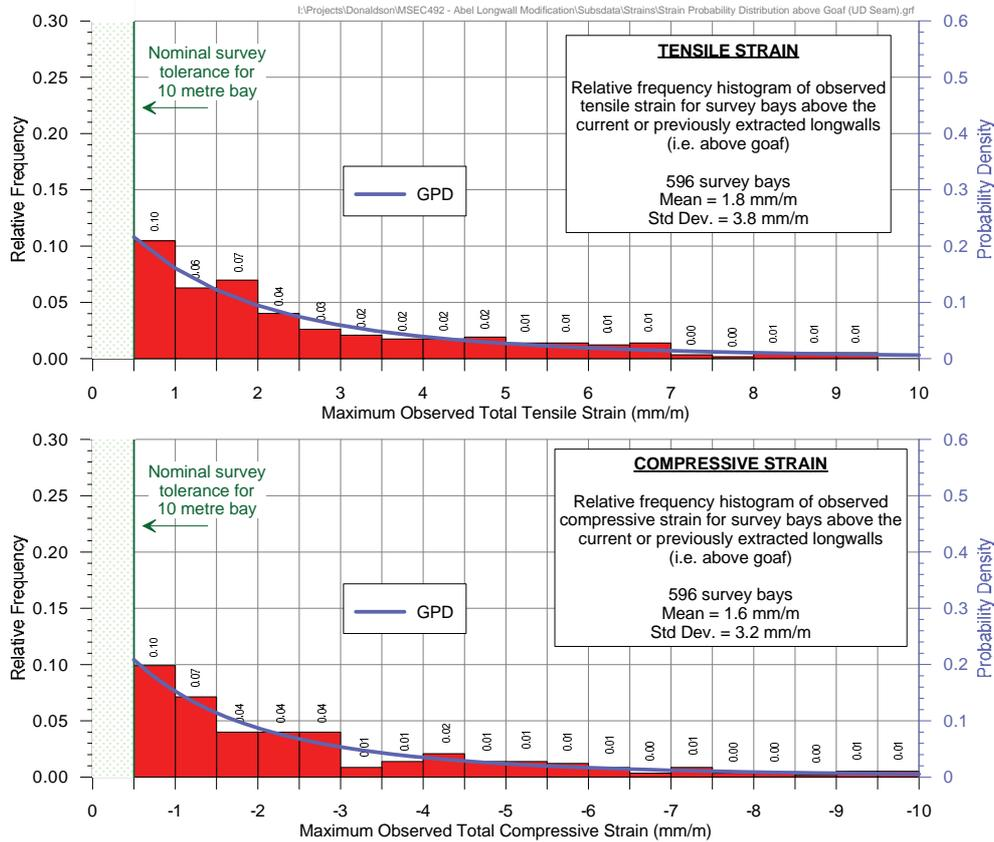
**Fig. 4.1 Distributions of the Measured Maximum Tensile and Compressive Strains in the Newcastle and Hunter Coalfields for Panels having W/H Ratios between 0.8 and 1.2**
