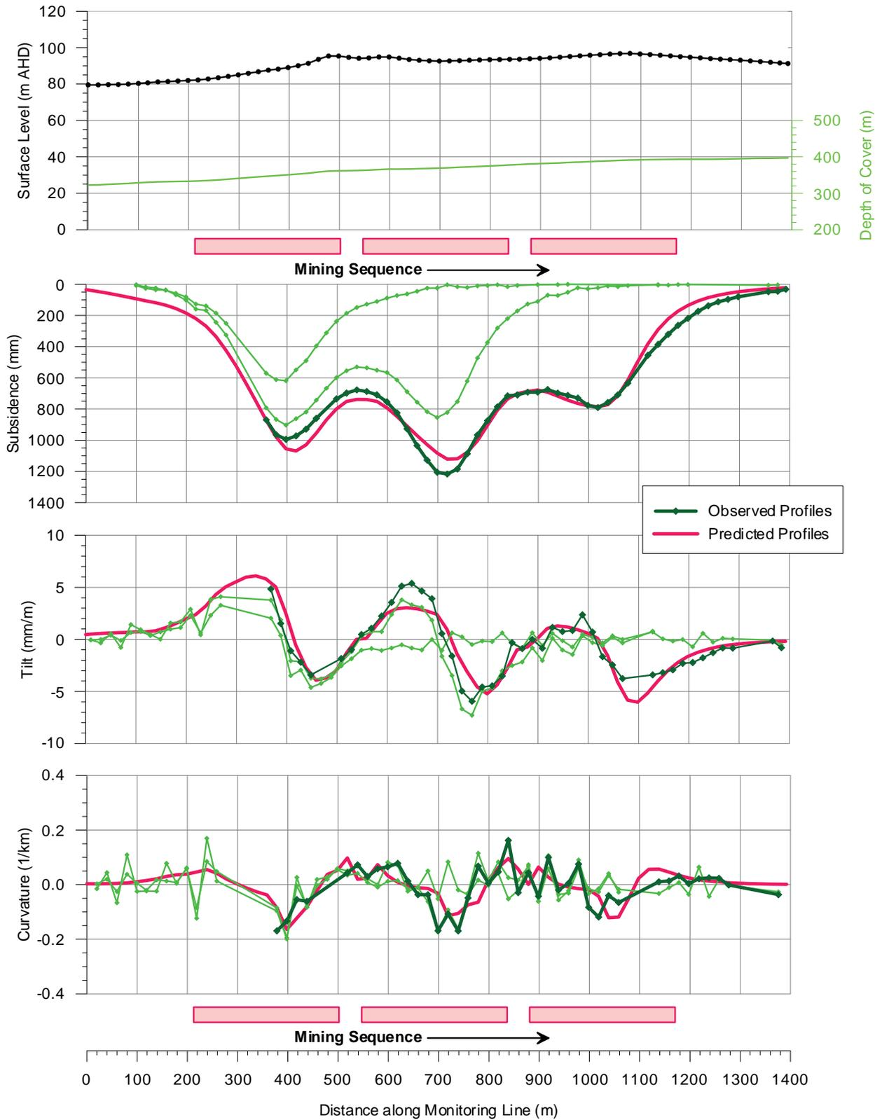
**Fig. 3.9 Comparison of Observed and Back-Predicted Subsidence, Tilt and Curvature along a Monitoring Line in the Hunter Coalfield with Panel W/H Ratio around 0.7**
