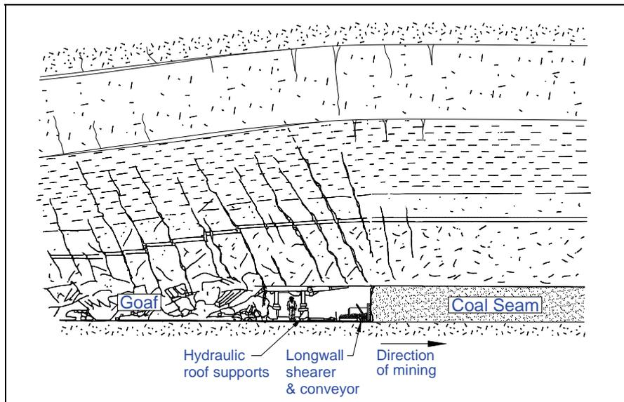
**Fig. 3.1 Cross-section along the Length of a Typical Longwall at the Coal Face**
