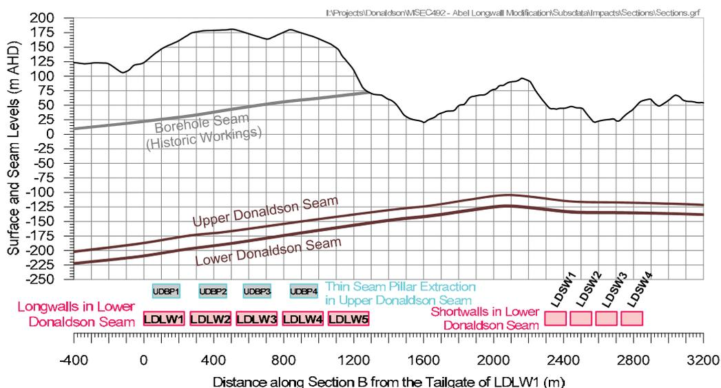
**Fig. 1.3 Surface and Seam Levels along Section-B (Thin Seam Pillar Extraction Panels, Longwalls and Shortwalls in Upper and Lower Donaldson Seams)**
