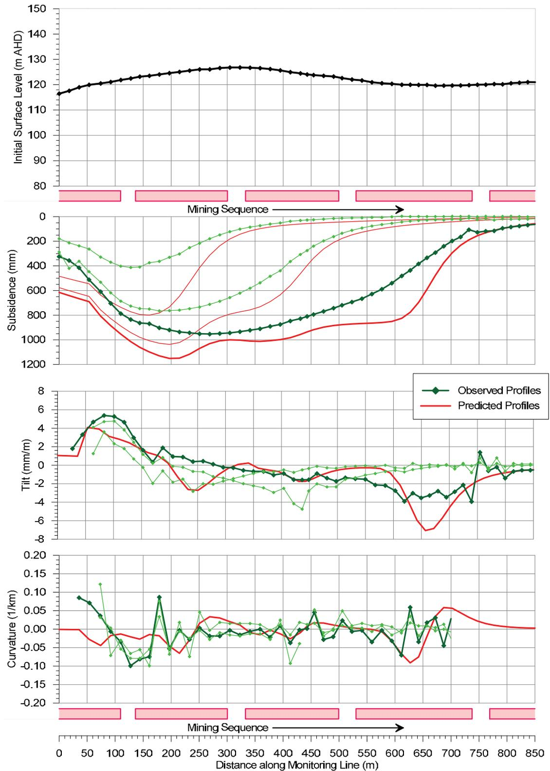
**Fig. 3.8 Comparison of Observed and Back-Predicted Subsidence, Tilt and Curvature along a Monitoring Line in the Newcastle Coalfield with Panel W/H Ratio around 0.4**
