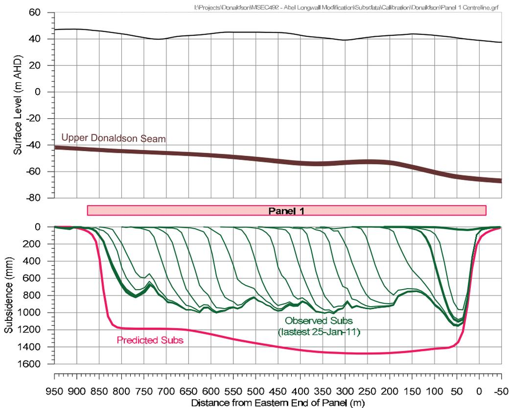
**Fig. 3.5** Comparisons between Observed and Back-Predicted Subsidence for Panel 1 Centreline
