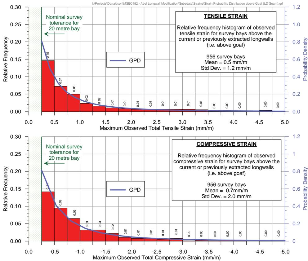
**Fig. 4.2 Distributions of the Measured Maximum Tensile and Compressive Strains in the Newcastle and Hunter Coalfields for Panels having W/H Ratios between 0.4 and 0.8**
