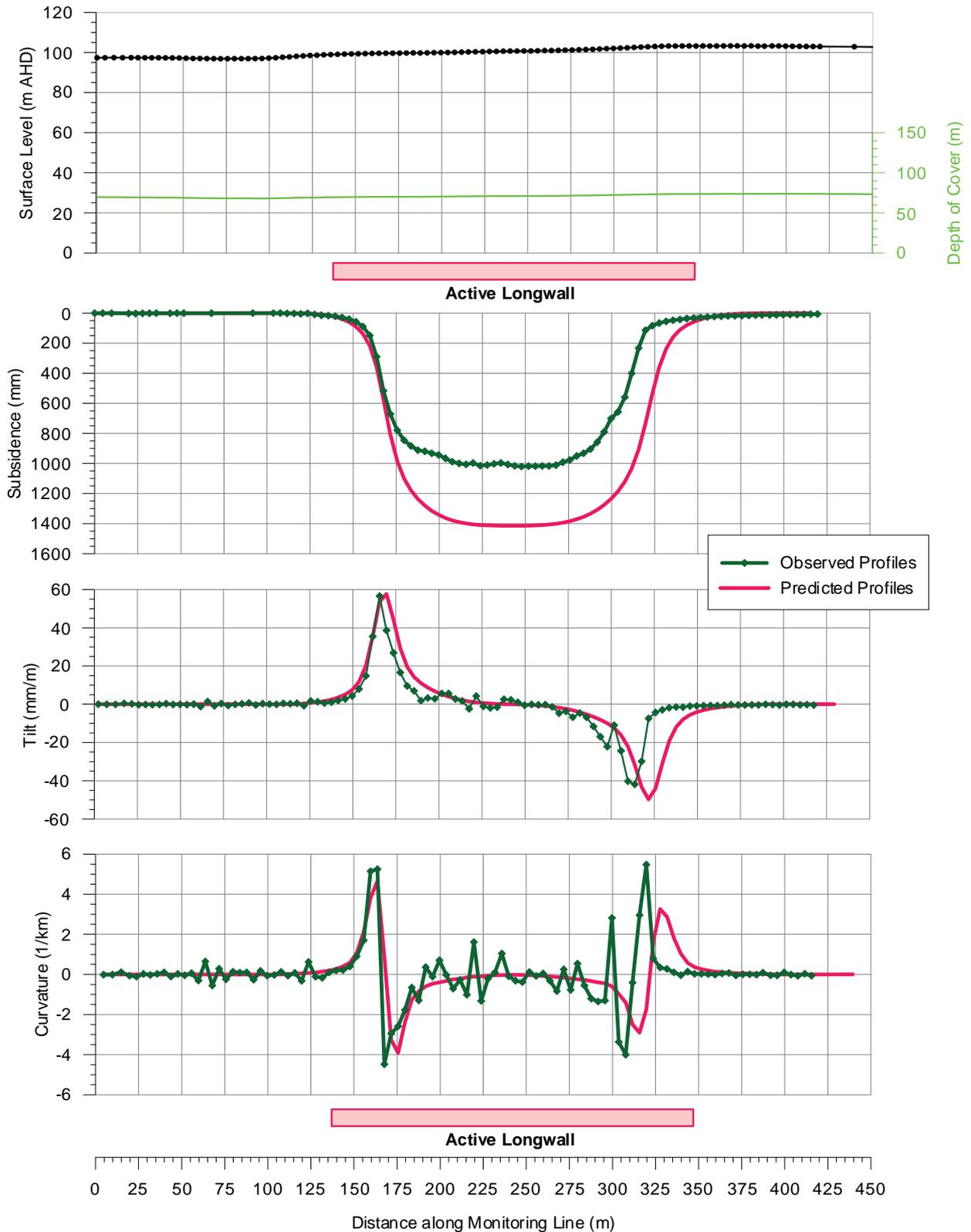
**Fig. 3.10 Comparison of Observed and Back-Predicted Subsidence, Tilt and Curvature along a Monitoring Line in the Hunter Coalfield with Panel W/H Ratio Greater than 2.0**
