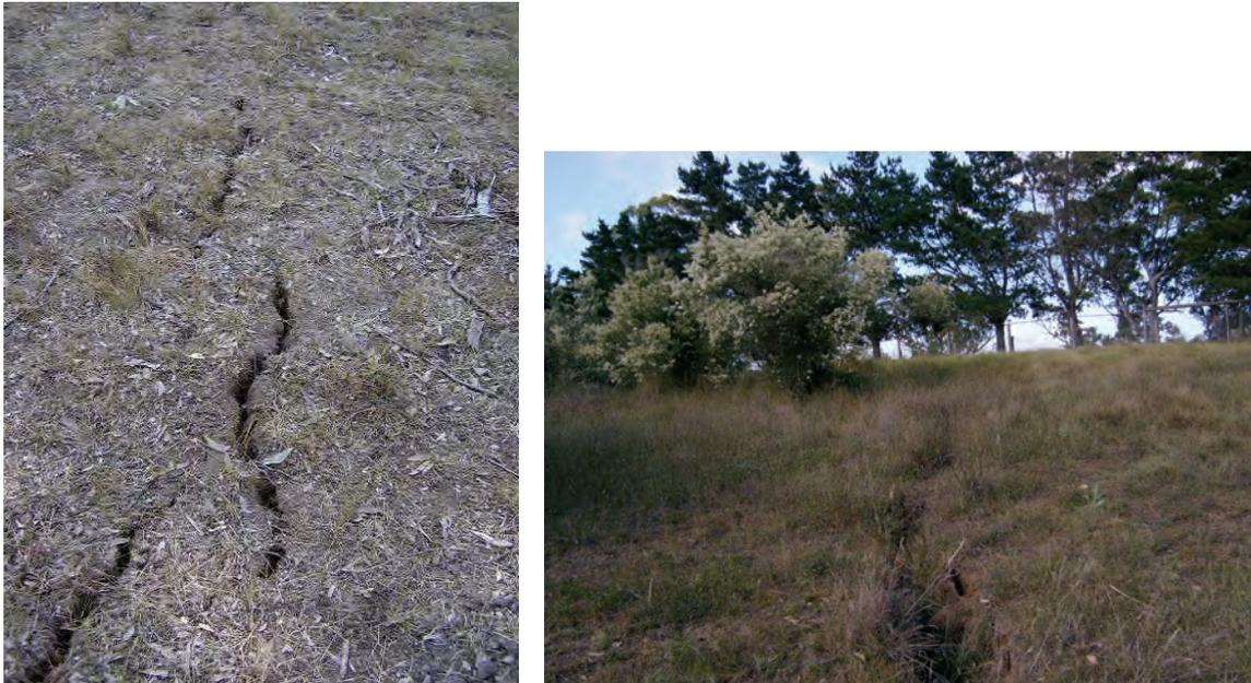
**Fig. 4.5 Photographs of Typical Surface Cracking in the Southern Coalfield (Greater than 400 metres Depth of Cover)**
