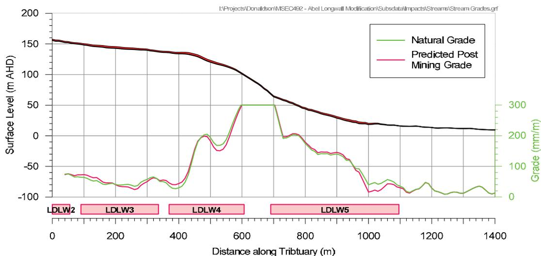
**Fig. 5.6 Natural and Predicted Post-Mining Levels and Grades along Tributary BGC1 Based on the Upperbound Subsidence Developing Above Proposed LDLW1 to LDLW5**
