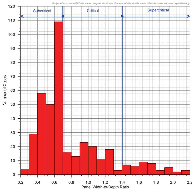
**Fig. 3.7 Distribution of Panel Width-to-Depth Ratio from the Empirical Database**
