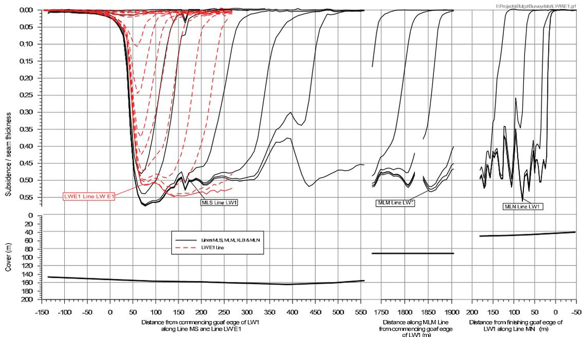
**Fig. 3.3 Observed Subsidence Profiles at South Bulga Colliery**
