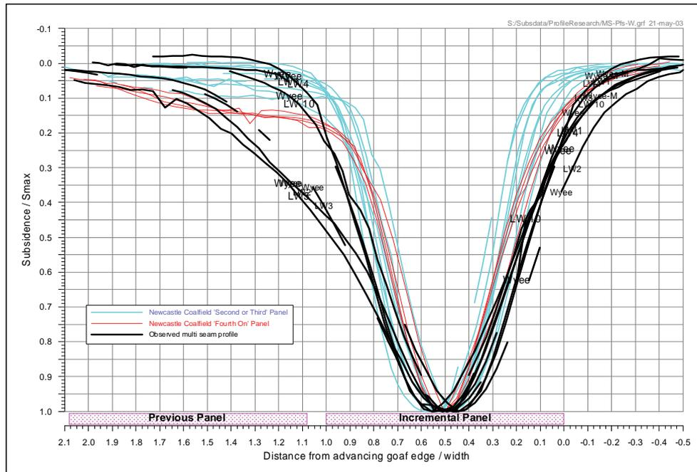
**Fig. 3.12 Comparison of Observed Single-seam and Multi-seam Subsidence Profiles**
