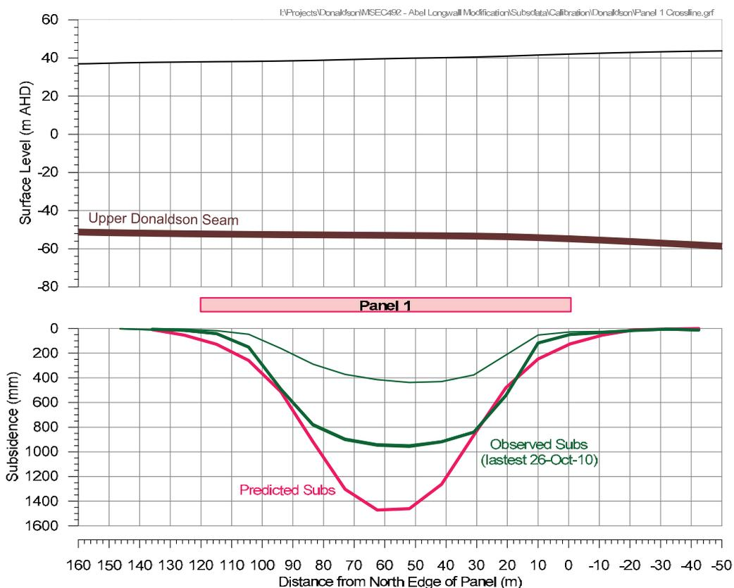
**Fig. 3.6** Comparisons between Observed and Back-Predicted Subsidence for Panel 1 Crossline
