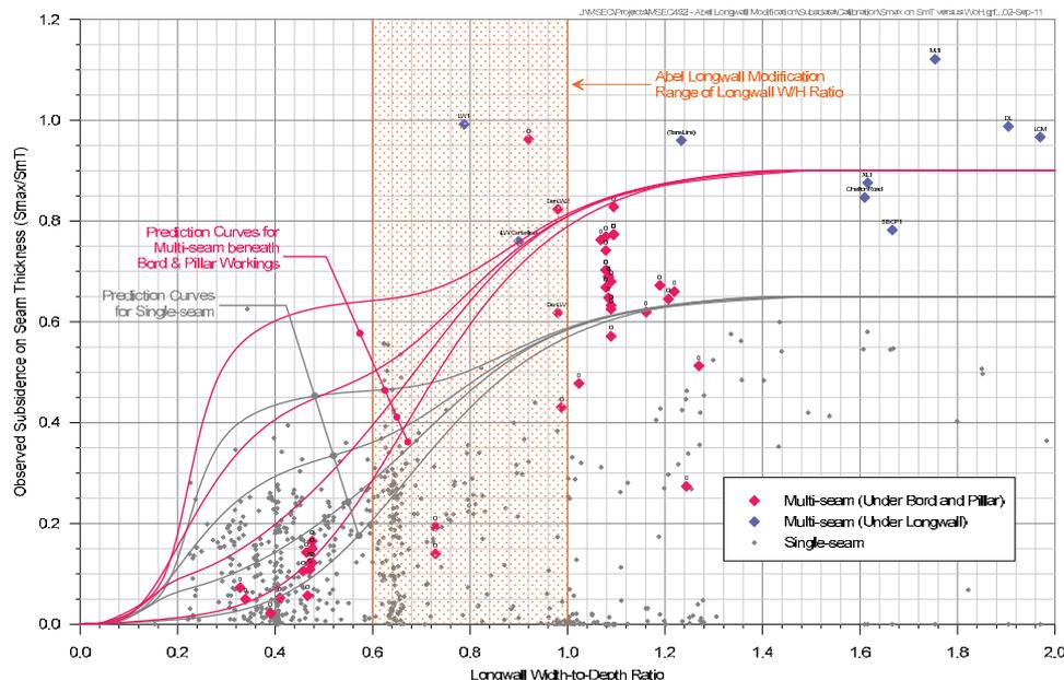
**Fig. 3.11 Maximum Observed Subsidence versus Longwall Width-to-Depth Ratio for Historical Multi-seam Mining Cases**
